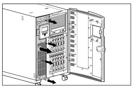
Figure 2-4. Removing the front fixed bezel
